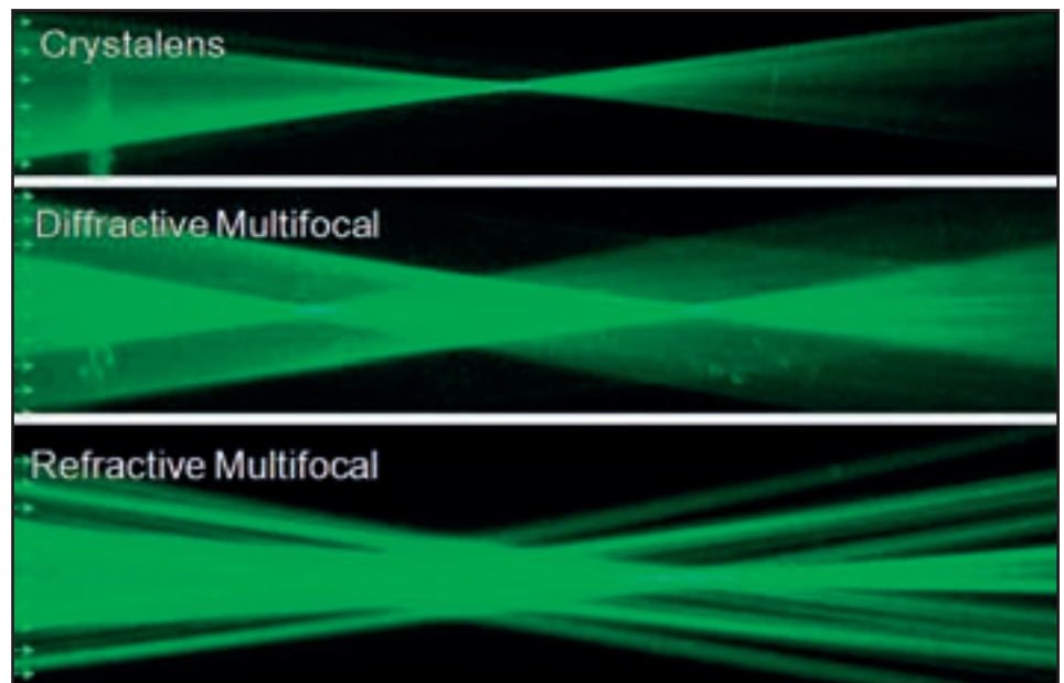
Ray tracing to compare the different presbyopia correcting lenses shows a single point of focus for the Crystalens as compared to multiple points of focus for the different types of multifocal IOLs
